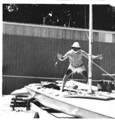
you will have a little play in step rope as mast angle ogets smaller that ok just don't look at it when all the way up slip mast into step, while holding mast forward uncleat step rope at foot of mast pick up safety rope and cleat it then advance to bow to hook up forestay
