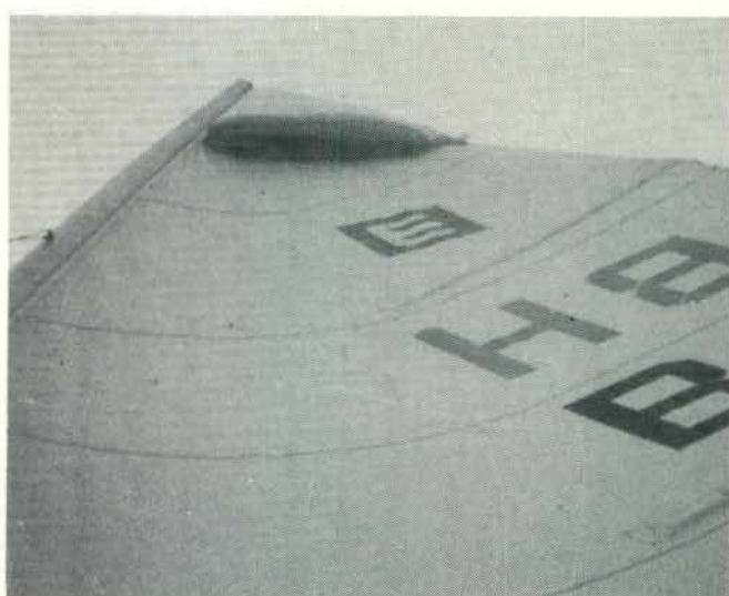
With wind above 7 mph, sailshape is excellent. Wrinkles in immediate area of foam and slight huckle there of the leech are only minor effects.
