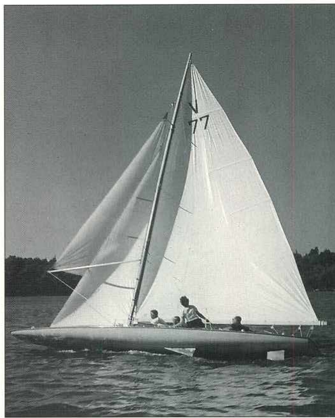
Stingray in the fifties - a family boat with wife Dede and son Hans; ILYA Champion 1953; apparent wind probably 50 degrees, an equilateral genoa without legal means forward of the mast line for forcing the luff to be tight. Mike designed the present block "E" in 1960, so that's what's missing in the picture. Stingray II was ILYA champ in 1963.
