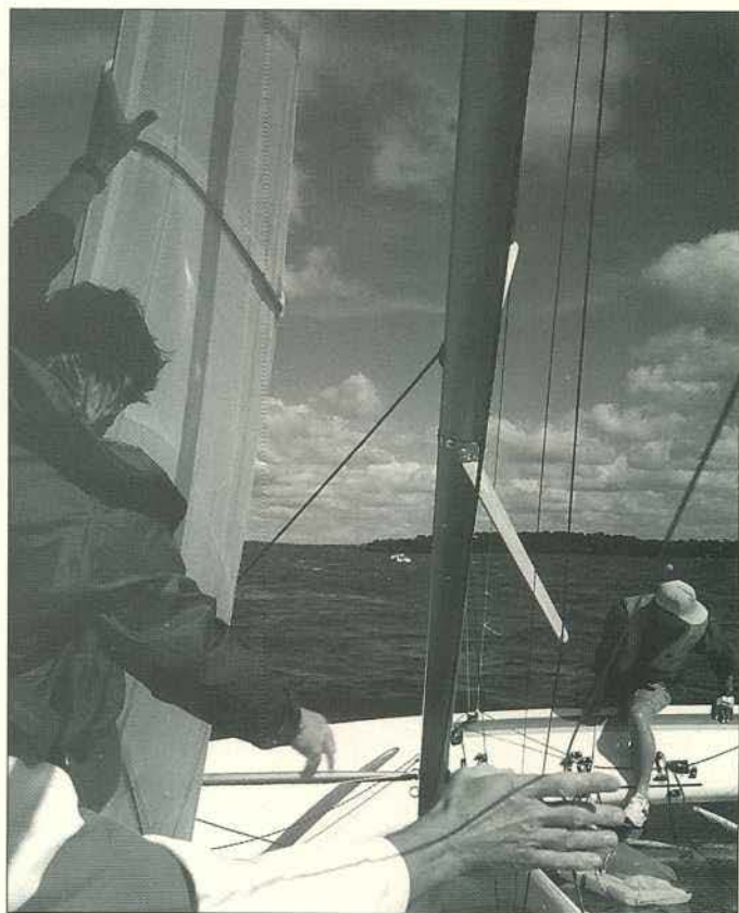
One way to right a scow is to walk the mast. The scow crew climbs in to the cockpit to stabilize the scow in the waves. Photo by Carolyn Stewart
